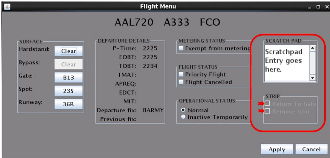
Figure 5.12. Scratch Pad, Return to Gate, Remove Icon.
